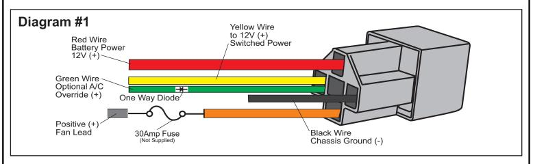
RED Wire - Attach to the Positive (+) Terminal of Battery
