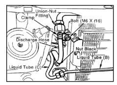
Locate and remove the condenser mounting bracket fasteners.
