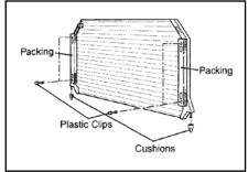
**NOTE:** Mounting hardware will vary by vehicle. Unless new mounting hardware is supplied or purchased, reuse the plastic clips, grommets, cushioning, brackets, spacers, bushings and hardware from the original condenser. Before installation, insert a piece of cardboard in front of the radiator to protect the fins.
