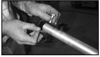
2a. Install new Sentry connecting clevis, using new washers, 1/2" bolts, and locknuts. Note: Excali-bar, and Aluminator use gray (thick) washers inside of clevis. Kwik-Tow uses white (thin) washers. Tighten 1/2" bolt so that there is a slight drag when pivoting clevis side to side. Note: On Kwik-Tow, long leg of clevis goes on top side of tube.
