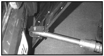
4. Slide right and left wings into Sentry connecting clevis until wings are approximately 1/4" away from bottoming out against clevis.
