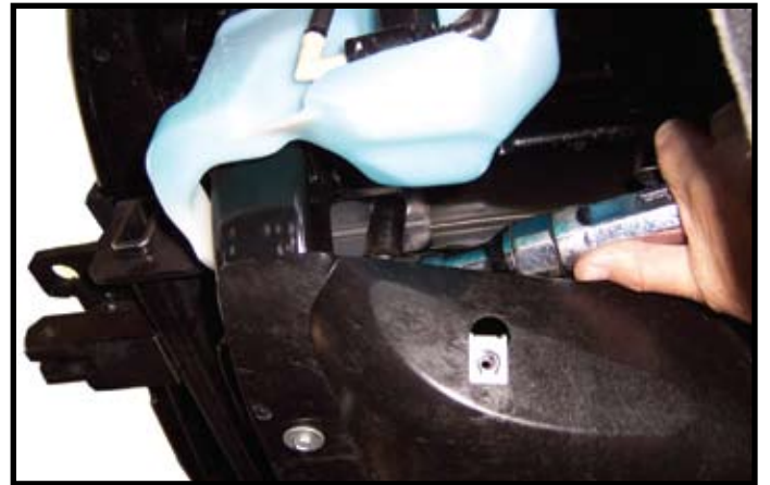
17. With an assistant, install baseplate up against bottom of frame. Fasten using four 10mm flat fender washers, 10mm lock washers and 10mm-1.50 x 35mm bolts, thread into existing threaded holes in frame, NOTE: Use blue LOCTITE® on all bolts and tighten all bolts according to chart on front page.
