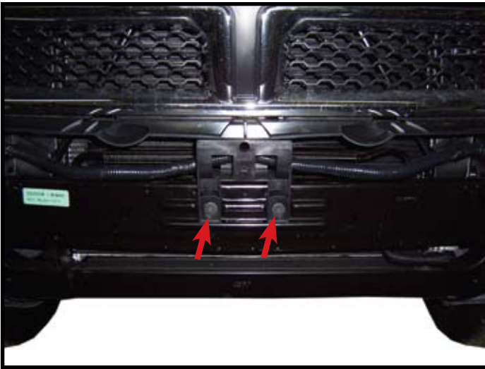
13. Remove two bolts from center grill support and remove support.
