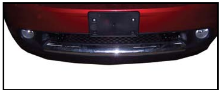
18. Reinstall air deflector, fascia and plug in fog lights. Use the plastic rivet instructions to install the supplied rivets to fascia.
