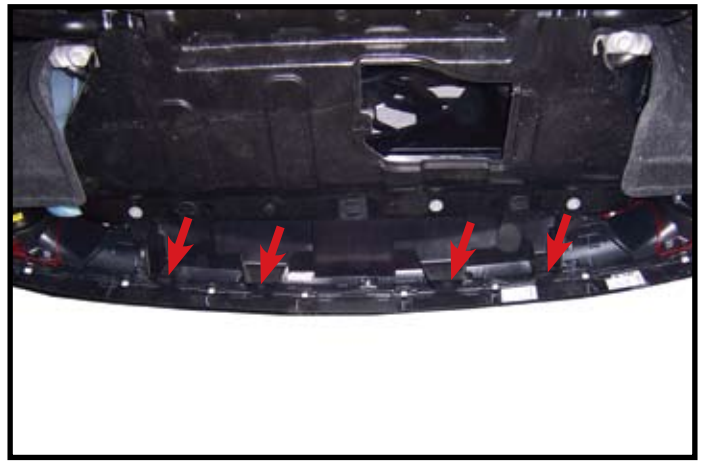
4. Remove four plastic push fasteners from bottom of fascia.
