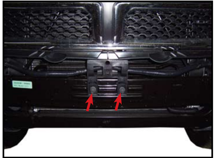
13. Remove two bolts from center grill support and remove support.
