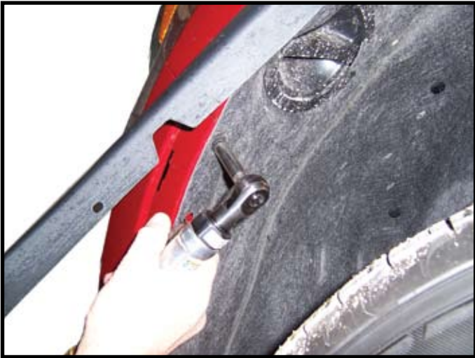
4. Remove one screw from fascia by trim molding.
