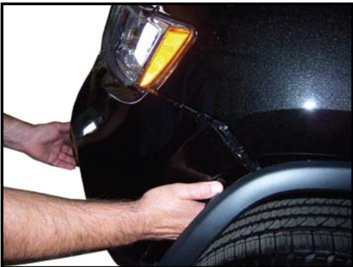
6. Carefully pull fascia out on each side by fender and pull fascia forward to remove. Unplug fog light if equipped.
