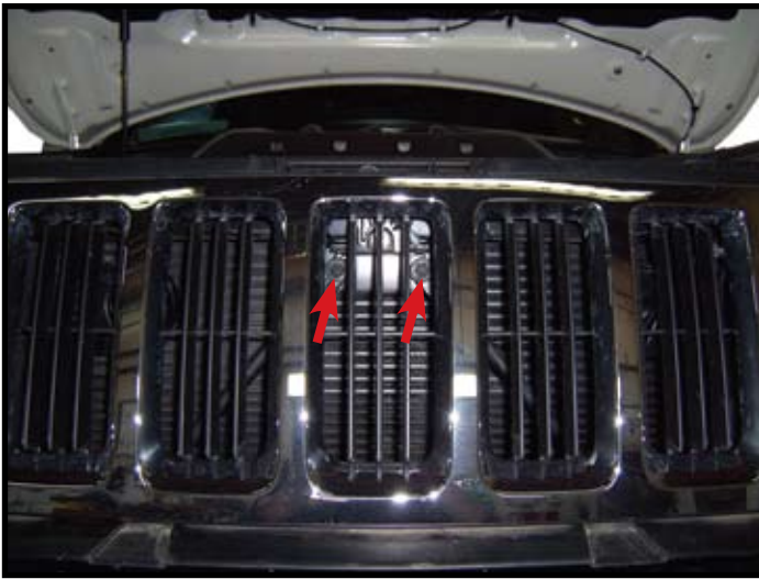
15. Remove two bolts from top bumper supports from behind grill. NOTE: Be careful not to damage radiator.
