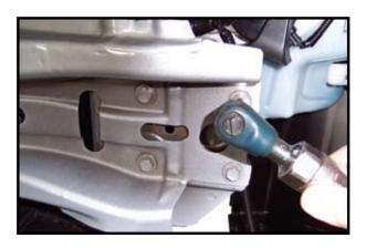
6. Remove four bolts from each side of the bumper and set bumper to the side. NOTE: If only three factory bolts are used, top inside two bolts will not be used. Step 10 is added to make up for 4th bolts.
