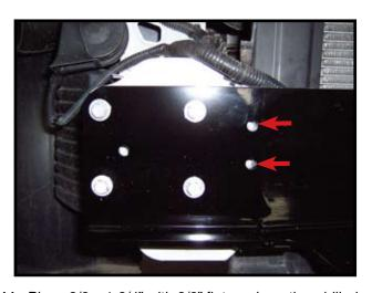
11. Place 3/8 x 1-3/4" with 3/8" flat washers thru drilled holes and place 3/8" flat washer, the 3/8" lock washer and 3/8" nut behind the bumper mount. NOTE: Use blue LOCTITE on all bolts and tighten all bolts according to chart on front page. Minor trimming of the bumper may be required to let the washers in the front Lay flat against the baseplate.
