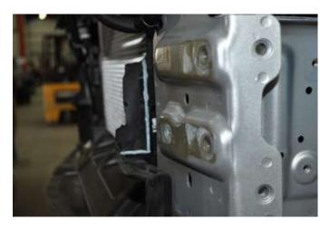
**8A. GMC Terrain:** Trim air damper as shown in picture, so baseplate can lay flat to mounts (both sides). Trim as needed.
