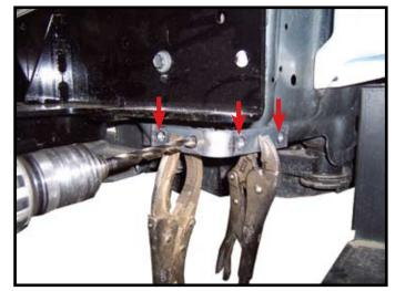
13. Clamp lower bracket to frame as shown. Make sure bracket is flush with bottom of pinch weld. Drill four 13/32" holes using bracket as a template. Repeat on other side.
