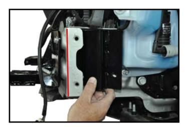
28. Install the driver side bracket in the same ways as on the passenger side. Follow step 22-25 for order of how to install bracket. NOTE: red line shows previously removed in Step 12.
