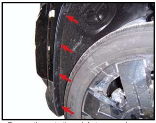
2. Remove three plastic push fasteners and one screw in the front of each fender well. Some models remove two plastic push fasteners and two screws.
