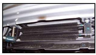
**5. If Equipped:** Remove the cooler from the bottom of the bumper and let hang. **Note:** bolts will not be reused.
