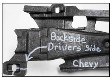
**31B. Chevy Equinox:** On the rear of the facia, cut the foam as shown above on each side.
