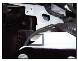
**17.** Cut frame above baseplate on each side as shown in picture. **NOTE:** Passenger side shown.
