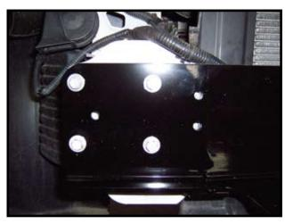
**9.** With an assistant, mount the baseplate into place with the bumper bolts.
