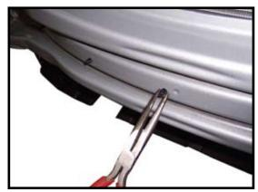
**4.** With a pliers pinch tabs that hold the wiring harness to the back of the bumper and let hang.
