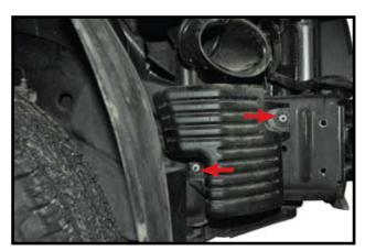
**22.** On passenger side remove the two nuts that hold the air box baffle in place. Remove baffle and set aside.
