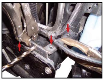
**18.** Clamp upper bracket to frame as shown. Make sure bracket is flush with the pinch weld on the side. Drill four 13/32" holes using bracket as a template. Repeat on other side.
