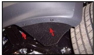
**3.** Remove two screws from the bottom of the facia on each side. Pull out firmly on outer corner of facia from the front of the fender. Unplug fog lights if equipped.
