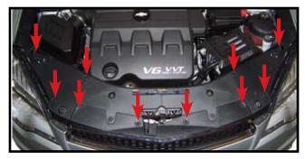
1. Open hood and remove 6 plastic push fasteners and 4 screws from the panel on top of the grill. Remove center plastic cover and hinge outer covers up and back. Lift outer panel to allow grill to be free.
