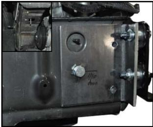
24. Insert 1/2"NC x 1-1/4" bolt and 1/2" lock washer through passenger side bracket and using a nutstrip on inside of frame through hole in bottom of frame as shown in corner picture (leave bolt loose for now). Place 8mm nut, 8mm lock washer, and 8mm flat washer on bolts that come through front of bracket and tighten. Once front nuts are tight then tighten 1/2" bolt. NOTE: Use blue **LOCTITE** on all bolts and tighten all bolts according to chart on front page.
