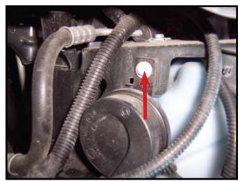
**16.** Remove one bolt on each side from horn and let hang.
