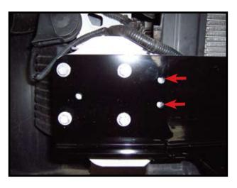
**10.** Drill two 13/32" holes using the baseplate as a template on each sides.
