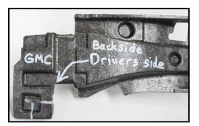
**31A. GMC Terrain:** On the rear of the facia, cut the foam as shown above on each side.
