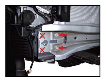
21. Remove factory bumper bolts and reinstall bumper using factory bolts in inside holes of bumper. **NOTE:** Use blue **LOCTITE** on all bolts and tighten all bolts according to chart on front page.
