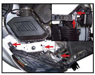
15. Remove three screws from the top of headlight assembly and two from the side (as shown in inserted picture). Pull headlight out and rest on engine. NOTE: Some headlights have a hidden tab holding light to fender. Headlight is removed for ease of drilling.
