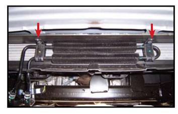
**30. If Equipped** Using the 1/4" x 1 bolts with flat washer and lock washers replace the cooler mounting it to the baseplate in the holes provided as shown.
