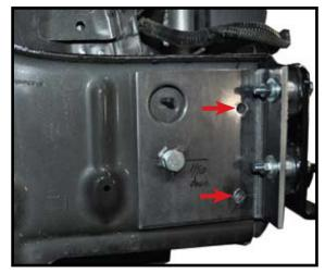
**25.** Drill two 13/32 holes through the outside of frame using the baseplate as a template.
