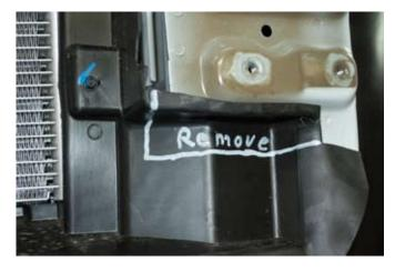
**8B. Chevy Equinox:** Trim air damper as shown in picture, so baseplate can lay flat to mounts (both sides). Trim as needed.
