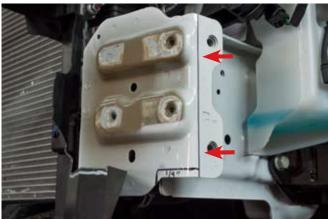
12. Cut frame below baseplate on each side as shown in picture. NOTE: Top picture reflects passenger side. Bottom picture reflects drivers side as this may be different. NOTE: vertical black line for cutting.
