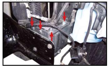
19. Place 3/8 x 1" bolts thru drilled holes and place 3/8" lock washer and 3/8" nut behind frame. NOTE: Use blue LOCTITE on all bolts and tighten all bolts according to chart on front page. Reinstall bolt holding horn on both sides.
