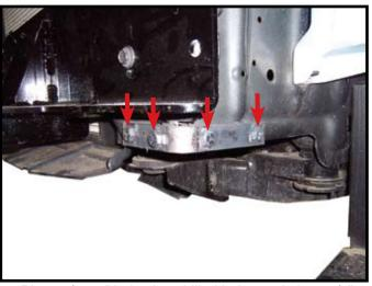
14. Place 3/8 x 1" bolts thru drilled holes and place 3/8" lock washer and 3/8" nut behind frame. **NOTE:** Use blue **LOCTITE** on all bolts and tighten all bolts according to chart on front page.
