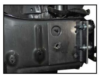
23. Place two bushings over the bumper mount nuts and place passenger side bracket tight to frame and bumper mount. Insert 8mm-1.25 x 50mm bolts, 8mm lock washers, and 8mm flat washers through bumper and passenger bracket. NOTE: Use blue ♣���TITF
