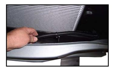
Route wiring as desired to prevent damage from harness
