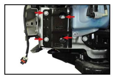
**7.** Remove four bolts from support bracket on driver side and remove. Bracket and bolts will not be reused.
