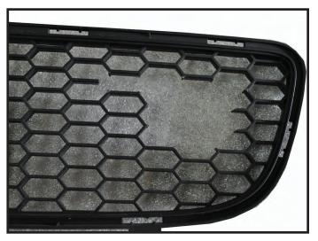
**11.** On each side of lower grill opening, trim as shown in picture. If needed trim fog light mount to allow facia to mount properly.
