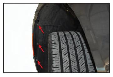
2. Remove three screws from front of each wheel well.
