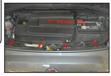
1. Remove four T30 Torx screws from top of facia.
