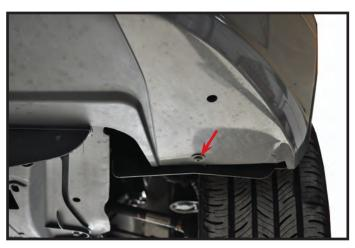
Remove one screw from facia in front of tire on both sides of vehicle.
