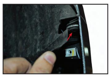
4. Remove one T30 Torx screw from behind inner wheel well liner on each side where facia attaches to fender.
