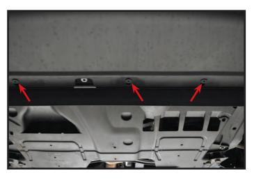
**5.** Remove three T30 Torx screws from underside of facia.
