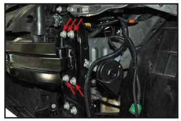
**8.** On each side of bumper remove four bolts and one nut and set bumper aside.
