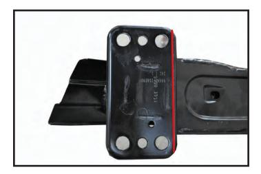
**9.** On each bumper mount remove material as shown by line in picture. Once material is removed slide over baseplate to make sure enough has been removed.
