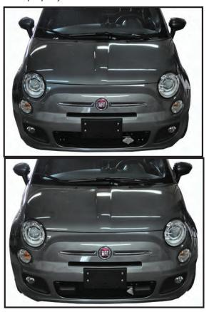
12. Reinstall facia in reverse order. Plug mount (item #7) may be installed if desired in convenience holes on either chain anchor or as desired. NOTE: Excess material may be trimmed from bracket.
