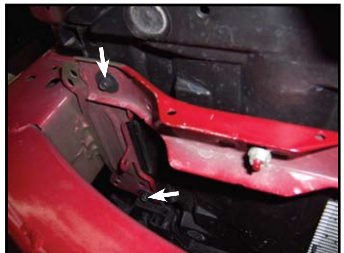
13. Remove two screws from each side holding radiator to bumper.
