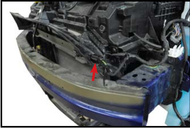
9b. 2014 Remove air temp. sensor from top of air deflector on drivers side.
