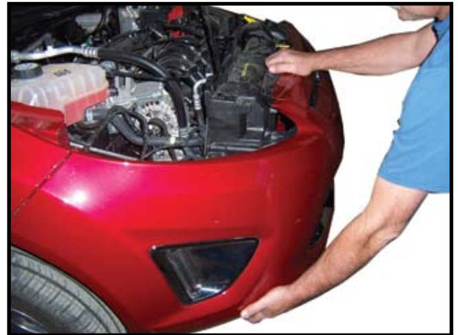
7. Remove fascia by pulling up and forward and unplug marker lights.
