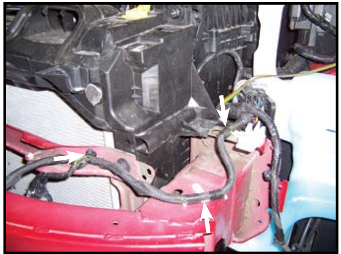
12. Remove several plastic push fasteners to remove wiring harness from bumper.
