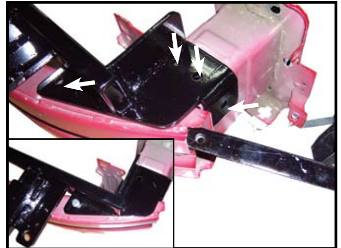
18. Line up slotted holes on each side and clamp baseplate to bumper. Use baseplate as a guide and drill front and side holes with a 13/32" drill. Insert nut strip in each side of bumper and fasten with 3/8" x 1-1/4" bolt and 3/8" lock washer. NOTE: Leave all bolts loose until later. Use blue LOCTITE on all bolts and tighten all bolts according to chart on front page.
