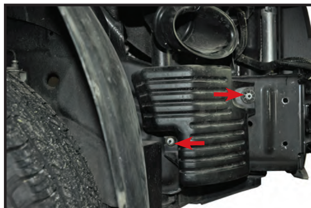
20. On passenger side remove the two nuts that hold the airbox baffle in place. Remove baffle and set aside.
