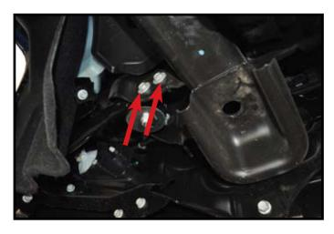
**4.** Remove two bolts from bumper side mount on out side of frame on each side of truck.
