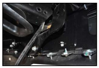
**7.** On the drivers side only take a bar and push the bumper forward far enough to remove front bolt. **NOTE:** This will also need to be done to reinstall bolt once baseplate pod has been inserted.
