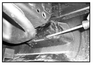
**2.** Remove tow hook plastic filler panels by releasing clips on filler panel from the back side of fascia. These will not be reinstalled.
