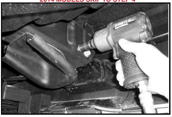
1. Remove tow hooks by removing two bolts from each tow hook. Longer bolt and nut will be reused when installing base plate. If you have no tow hooks use item #8, #9, and #10.
