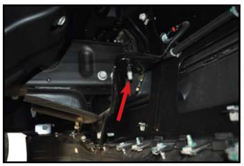
**5.** Remove one bolt from center bumper mount on inside of frame on each side of truck.
