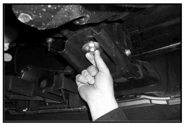
**9.** Install supplied 1/2" x 2" hex bolt, 1/2" lock washer, 1/2" frame washer, and tighten all bolts.
