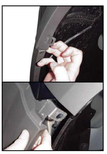
**5.** Pull facia straight down by fender, and release tab on facia (see pictures). Carefully pull facia forward and off.
