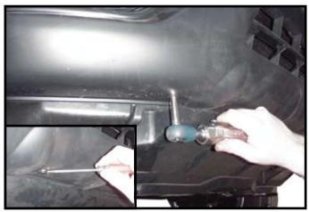
2. Remove two bolts from each side from bottom of facia on outside edges and two plastic push fasteners from center, underneath facia front.
