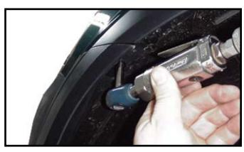
**3.** Remove one screw from each side, facia to fender, by going through wheel well.
