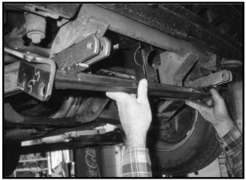
Position base plate on vehicle with center upright mount in the center of subframe cross tube.
