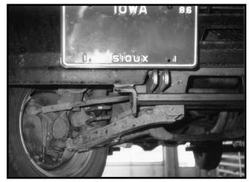
**5.** Thread four 3/8" x 1-1/4" hex head bolts with lockwashers, through base plate and frame, into nut plate. Tighten all bolts to specified torque on front page.
