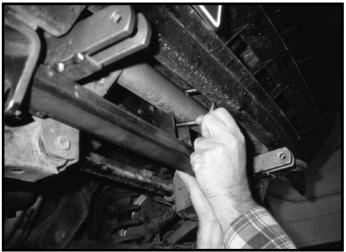
2. Secure base plate on vehicle using a 3/8" x 2-1/8" round u-bolt, lockwashers and hex nuts. Snug tighten u-bolt. Always use "LOCTITE. Blue" on threads.
