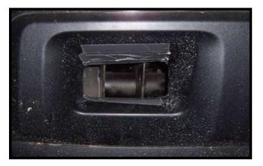
**2.** Apply protective tape (duct tape) by lining top and bottom of tow hook opening to protect facia during installation.
