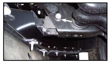
3. Slide base plate pull pods into end of frame. (See front page for which pull pod is passenger side and driver side.) Insert long cross bolt now and check for alignment of baseplate bottom bolt thru frame. In some cases this hole may have to be slightly elongated with a die grinder.
