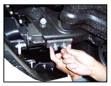
4. Install back-up plate with two 1/2" UNC 1-3/4" bolts, 1/2" lock washers, and 1/2" flat washers. **NOTE:** One side of back-up has a washer welded on, this will go into large hole in frame.
