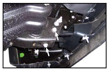
Remove tow hooks, on each side, by removing two bolts from each hook. NOTE: Long cross bolt and nut will be reused.
