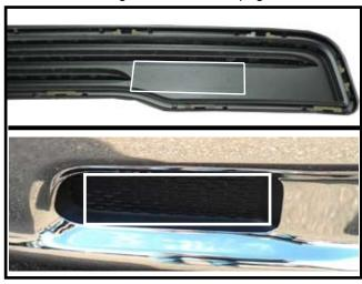
**11.** Trim bumper center insert as desired for finished look and reinstall (see top picture). Refer to bottom picture if not equipped with tow hooks.
