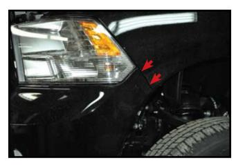
**5.** Remove facia by pulling down to release plastics studs then forward.
