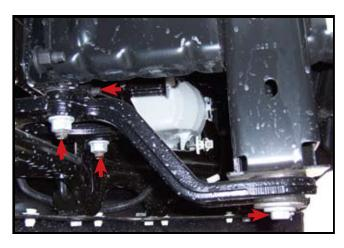
6. If equipped with tow hooks remove three bolts that hold the hook and remove the three nuts from the bumper and remove brackets. NOTE: The hook, brackets and the three bolts will not be reused.
