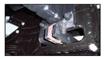
**9.** Place pull pod on the 3 bolts studs and replace 3 nuts leaving nuts loose Repeat steps 3, 4 ,5 and 6 for opposite side.
