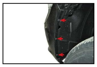
1. Remove one screw and two plastic screw fasteners from each wheel well in front of tire.
