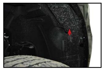
2. Remove one plastic push fastener from each inspection flap in front portion of each wheel well.
