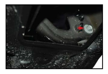
**3.** Inside of each inspection hole remove one bolt that attaches the facia to front fender.
