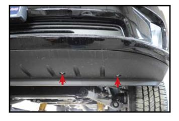
Remove two screws from each side from bottom of facia.
