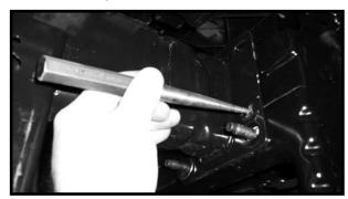
4. Flatten raised tab with a hammer and punch.
