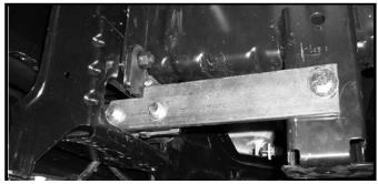
7. Attach rear brace on back of each pull pod using two 3/8" x 1-1/2" bolts, two 3/8" washer and two 3/8" lock washer connecting it to frame with one 7/16" x 5-1/2" bolt ,one 7/16 lock washer and one 7/16" flat washer and 7/16" nut and tighten all bolts. Use blue **LOCTITE** on bolts and tighten all bolts according to chart on front page.
