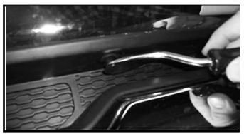
1. Remove Center bumper insert by removing six plastic push fasteners.
