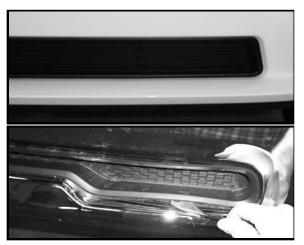
2. Gently pry around insert to release tabs on back side.
