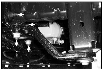
3. If equipped with tow hooks remove three bolts that hold the hook and remove the three nuts from the bumper and remove brackets. **NOTE:** The hook, brackets and the three bolts will not be reused.
