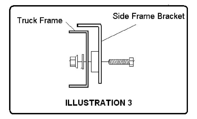
7. Tighten all bolts according to **BOLT TORQUE SPECIFICATIONS** chart. Failure to tighten bolts according to chart may result in fastener loss or failure.
