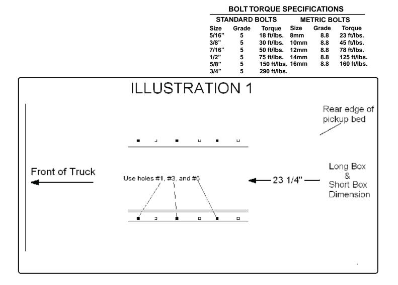
**CAUTION:** Do not install base rails over plastic bed liners. Plastic bed liners must be cut out of the way. Rails may be installed on spray in liners.
