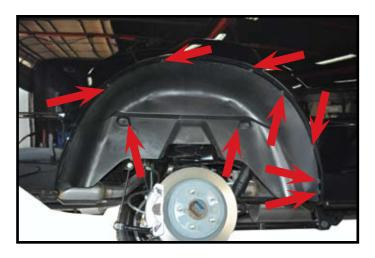
Remove remaining nine screws from each wheel well insert.
