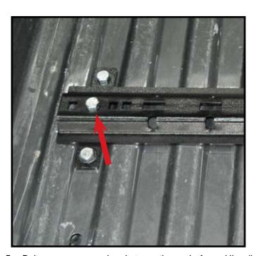
5. Bolt on rear spacer brackets on the end of one UL rail (bed rail) using 5/8" x 1 1/2" Gr.5 bolt. Apply included LOCTITE® to these bolts and tighten making sure that brackets are square with the UL rail. NOTE: Brackets bolt to the second hole from the end as displayed in above picture.. This rail will be the back rail you will measure to in the next step.
