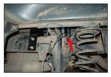
**10.** Repeat above directions for middle frame bracket. Clamp loosely to coil tower framework and tighten.
