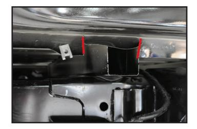
5. Cut flange as shown in each side in picture by box support behind coil spring. **NOTE:** Be careful to not heat up the box paint may discolor in box.
