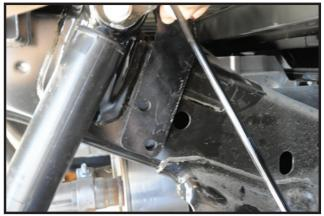
Slide front frame brackets to outside of frame and mount front bed rail while keeping frame bracket tight to frame. Tighten all bed rail bolts according to chart on front page. Passenger side shown.
