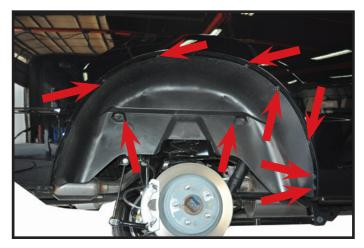
4. Remove remaining nine screws from each wheel well insert.
