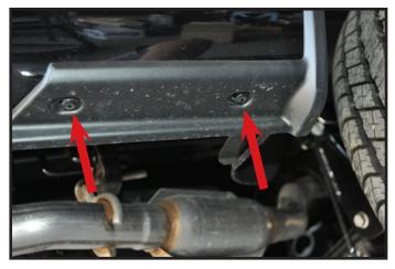
2. Remove two plastic push fasteners from bottom of box as shown in picture. Repeat on other side.
