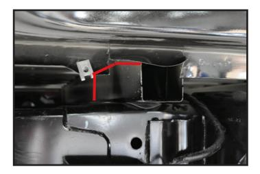
6. On the back side of box support cut along top and 7" in from end and then down. Fold back of support down and make bottom of box flush for clearance for frame bracket.
