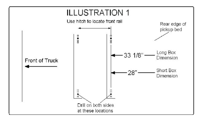
**CAUTION:** Do not install base rails over plastic bed liners. Plastic bed liners must be cut out of the way. Rails may be installed on spray in liners.
