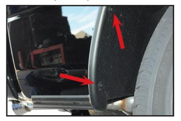
3. Remove two screws from plastic trim behind each wheel as shown.
