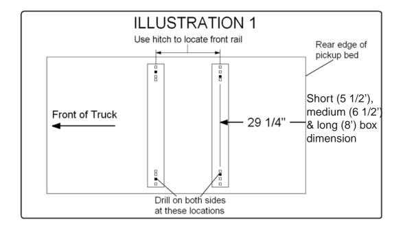
**CAUTION:** Do not install base rails over plastic bed liners. Plastic bed liners must be cut out of the way. Rails may be installed on spray in liners.
