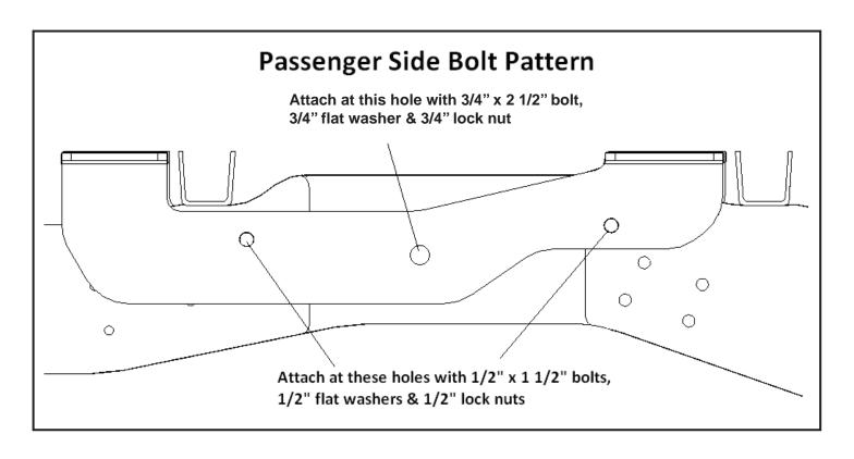
7. Each of the frame brackets must be attached to the side frame of the truck with a 1/2" x 1-1/2" hex bolts (01254) and 1/2" x 1-3/4" knurl bolt (14266) (drivers side only) at the for ward and rear holes and a 3/4" x 2-1/2" (05047) hex bolt in the middle hole. See Illustration 3.
