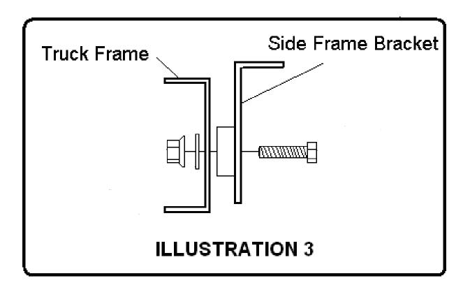
8. Tighten all bolts according to chart on front page. Failure to tighten bolts as described may result in fastener loss or failure.
