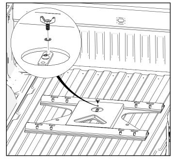
2. Lower frame adaptor into the factory pucks. Make sure the frame is fully placed into the pucks. Turn locking turn plate 1/4 turn so it is facing front to back and the locking holes line up. Install and tighten 1/4" internal tooth lock washer and 1/4" thumb bolt to secure locking turn plate into place. Lift up on frame to make sure it is securely fastened.
