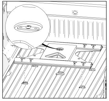
1. To install the adapter, remove the bed puck covers if installed. Turn locking turn plate so it is facing side to side as shown.
