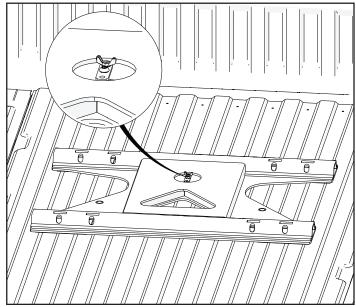
**4.** Install and tighten 1/4" internal tooth lock washer and 1/4" thumb bolt to secure locking turn plate into place. Lift up on frame to make sure it is securely fastened. Reverse steps to remove.
