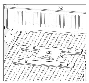
**3.** Install and tighten 1/4" internal tooth lock washer and 1/4" thumb bolt to secure locking turn plate into place. Lift up on frame to make sure it is securely fastened. Reverse steps to remove.
