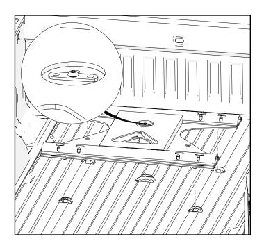
1. To install the adapter, remove the bed puck covers if installed. Turn locking turn plate so it is facing side to side as shown.
