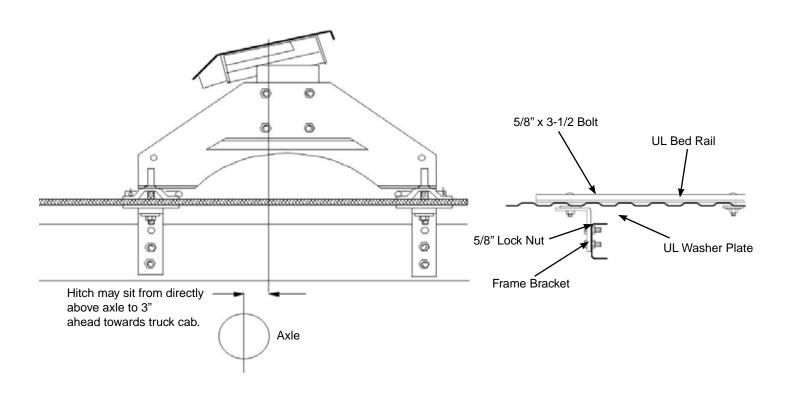
**IMPORTANT NOTICE:** This installation may require different frame brackets for the various truck models. This kit does not contain any frame brackets for this reason.
