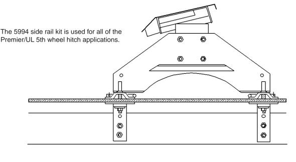
Install bedrail pull pins from under the side rail so that the hitch pin secures in the open.
