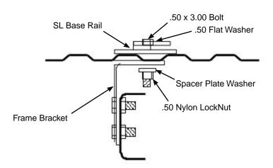
**IMPORTANT NOTICE:** This installation may require different frame brackets for the various truck models. This kit does not contain any frame brackets for this reason.
