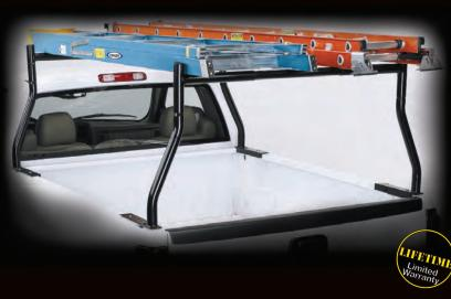
A pair of these high-strength racks will support up to 500 pounds of cargo. Long mounting plates provide stability without horizontal connecting bars between the two racks. The free-standing racks provide a wide area for easy access to load and unload bulky cargo from the sides. a crossover truck box can be mounted flush against the front rack creating more free space in the bed.
