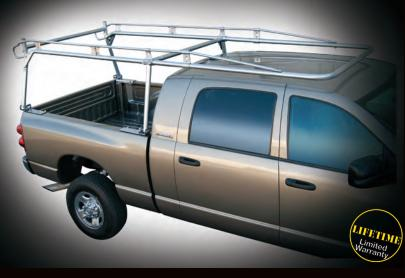
Swaged joints and fully gusseted crossbars for superior load capacity and the abrasion and corrosion resistant polyester marine-grade ClearCoat powder paint finish make the PRO IV Aluminum Ladder Rack a perfect choice. Triple-plated fasteners with chrome plating over double nickel plating.
