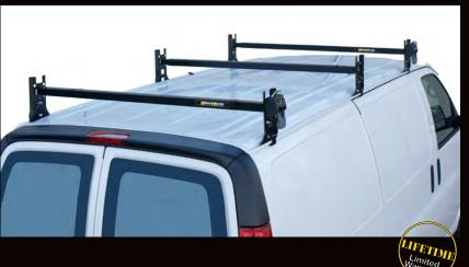
High-strength 1-5/8" diameter telescoping steel racks adjust to fit different width fullsize vans with rain gutters. Heavy-duty mounting brackets allow positioning the cross bars at different heights to provide proper clearance and reduce wind noise. EZ-mount Clamps secure the brackets on the rain gutters. They are easy to install or remove. Use 3-Bar Rack for more support of longer or heavier loads.
