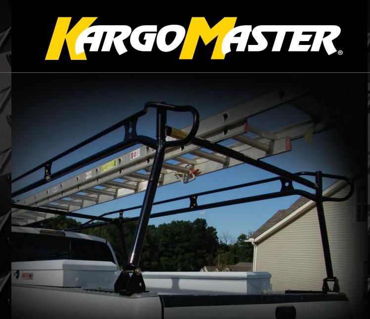
KargoMaster offers commercial-duty truck and van racks that are easy-to-install and adjust to your custom needs. All the racks have a yellow zinc dichromate undercoat and tough marine-grade powder coat epoxy finish for superior corrosion resistance and long-term durability. With a full breadth of truck and van racks and accessories, KargoMaster delivers superior fit, durability, and maximum convenience. Plus they have Lifetime Frame Warranty.
