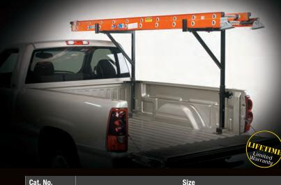
Quick Pac Racks are easy to insert in the mounting bases when needed and simply lift out of the bases until needed again. They can also be left in the bases permanently. The side-mounted racks support 250 pounds and are ideal for occasional use or when a full-length or heavier-duty rack is not required. Width of the racks adjusts from 18" to 32" to support different types and sizes of cargo.
