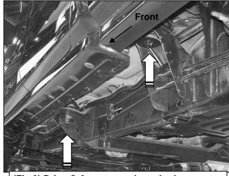
(Fig 3) Driver/left center and rear body mounts
