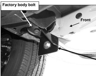
(Fig 3) Passenger side front Bracket pictured
