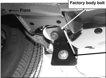
(Fig 3) Passenger side front Bracket pictured
