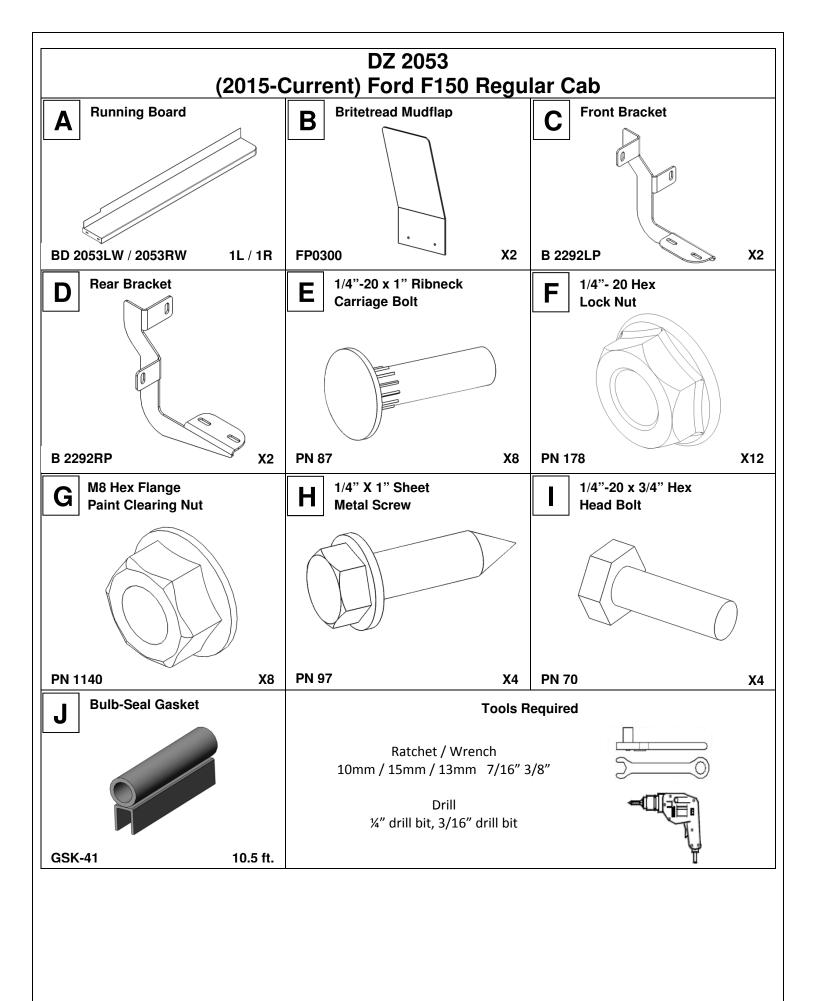
Cut each Bulb Seal Gasket (J) into two pieces, with one piece being 7 inches and the other piece being 55 inches. Assemble each running board using one Brite-Tread Running Board (A), one 55 inch piece of Bulb Seal Gasket (J), one 7 inch piece of Bulb Seal Gasket (J), one Brite-Tread Mud Flap (B), two 1/4"-20 X 3/4" Hex Head Bolts (I), and two 1/4"-20 Hex Lock Nuts (F).
