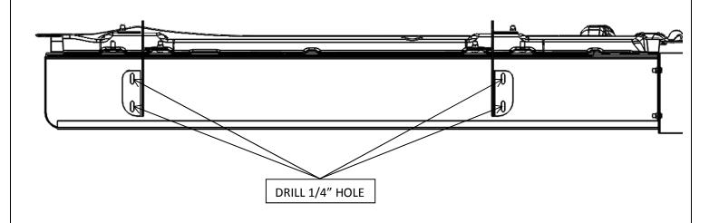
Attach the Brite-Tread Running Board to the braces using four 1/4"-20 X 1" Carriage Bolts (E) and four 1/4"-20 Hex Lock Nuts (F). Tighten using a 7/16" wrench or ratchet.
