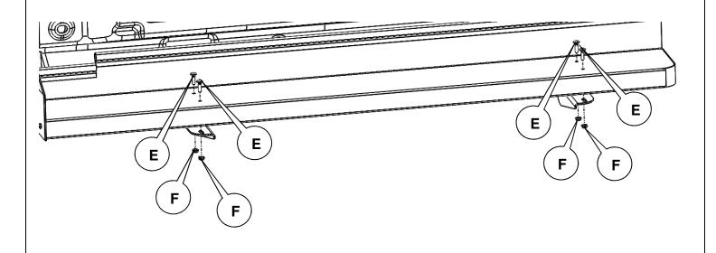
Attach the Mud Flap (B) to the wheel well by drilling two 3/16" holes using a drill through the mud flap and wheel well at the approximate locations as shown. Insert two 1/4" x 1" Sheet Metal Screws (H) and tighten using a 7/16" wrench or ratchet.
