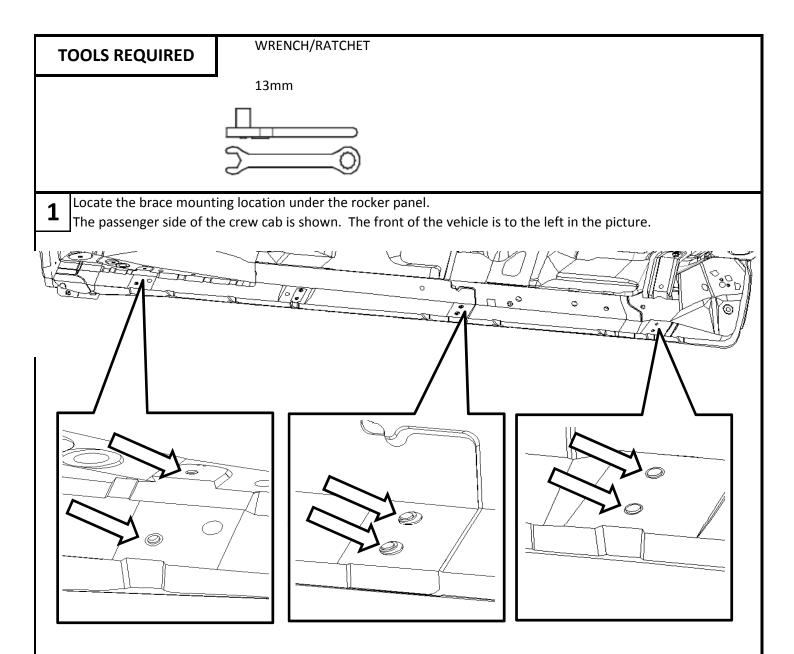
The regular cab will only have 2 mounting location. It will use the front and middle brace. For regular cab installations, the rear brace can be discarded.
