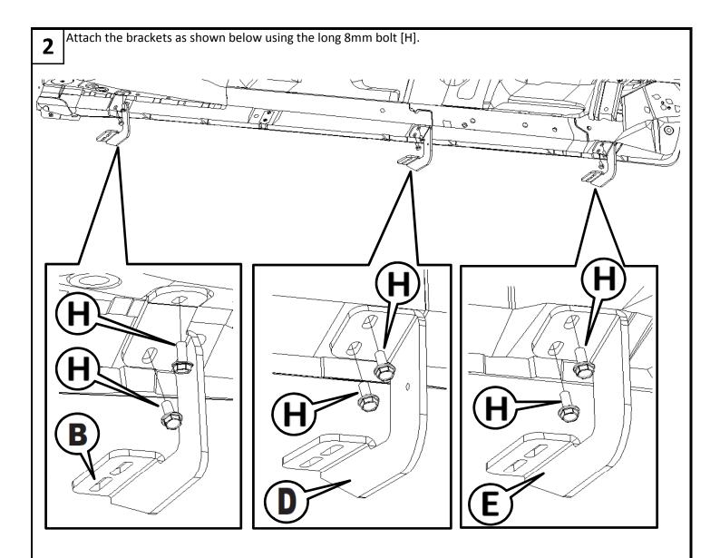
Tighten bolts with a 13mm Socket or wrench.
