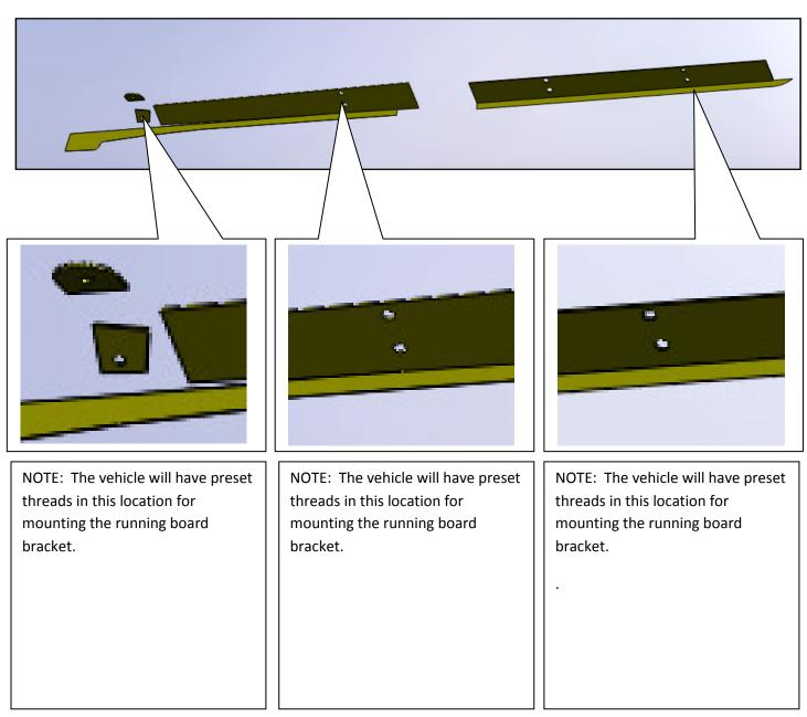
NOTE: FOR STANDARD CAB APPLICATIONS, THE MIDDLE BRACES (D & E) WILL BE USED AS THE REAR BRACE. THE STANDARD CAB WILL ONLY USE 2 BRACES PER SIDE, THEREFORE BRACES F & G MAY BE DISCARDED.
