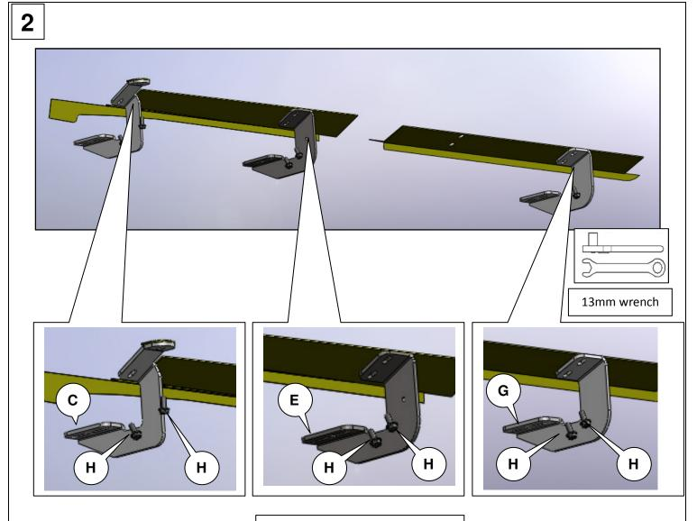
NOTE: THE MIDDLE BRACKET CONTAINS AN IDICATIOR HOLE TO DIFERENTIATE FROM REAR BRACKET.
