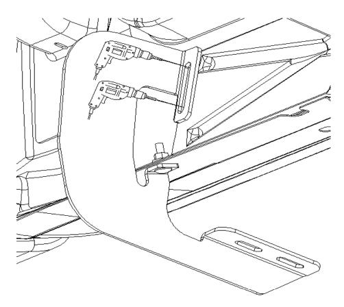
Attach the brace with two sheet metal screws [F] using a 3/8" wrench/socket.
