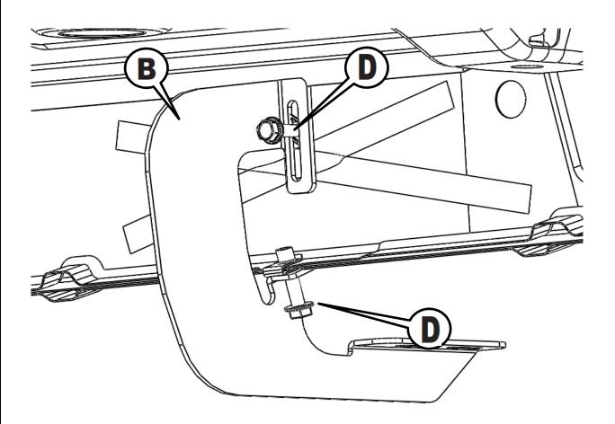
Tighten bolts with a 13mm Socket or wrench.
