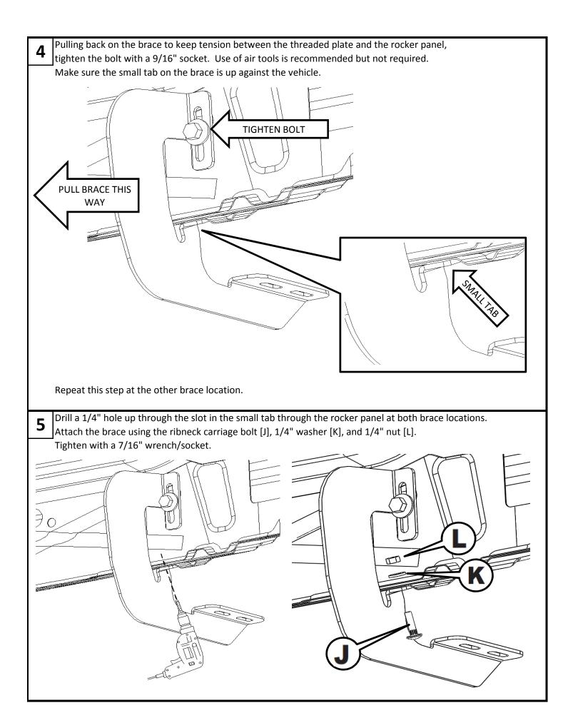
The next two steps are for the rear brace on the extended and crew cab pickup only. For the extended cab, measure back from the middle brace 20".
