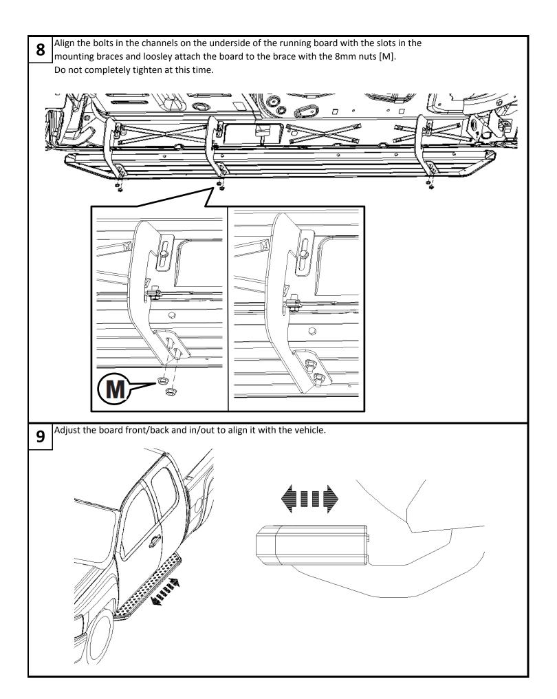
Once the board location has been set, tighten the nuts holding the board to the braces using a 13mm socket/wrench.
