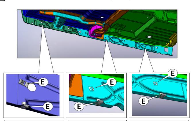
NOTE FOR 2007-2013: Your 2WD vehicle may not any preset fasteners in the hole patterns shown. If this is the case, use additional u-nuts (ITEM "E") to install in all locations as necessary.
