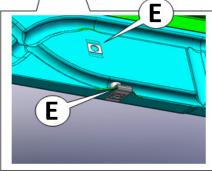
NOTE FOR 2007-2013: Your 2WD vehicle may not any preset fasteners in the hole patterns shown. If this is the case, use additional u-nuts (ITEM "E") to install in all locations as necessary.
