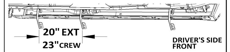
Hold the brace against the inner rocker panel and pinch weldl. Mark the slot in the small tab and drill a 1/4" hole through the rocker panel.
