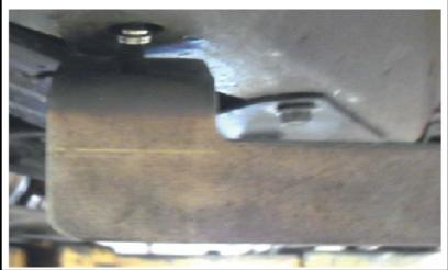
Note: If your vehicle is equipped with the optional skid plate package, one of the skid plates will be covering the mounting hole for the small threaded plate. This skid plate will need to be removed to allow access to this mounting hole.
