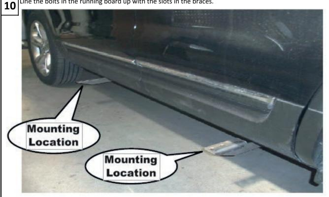
Place the board on the braces with the bolts through the brace slots.
