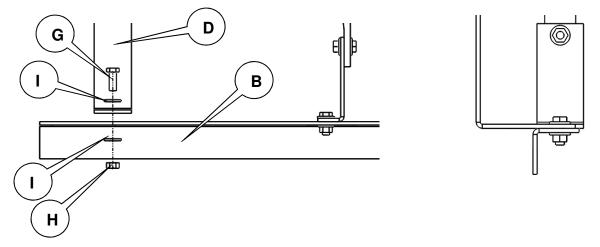
At the front Driver's Brace Location, attach the top of Frame Bracket (E) to the undercarriage panel as shown below using one 1/4"-20 X1" Bolt (G), two 1/4" Washer (I), and one 1/4"-20 Nut (H) using a 7/16" Wrench or Ratchet. Use a level to make sure that the Angle Brace (C) is parallel to the ground. Do not completely tighten at this time.
