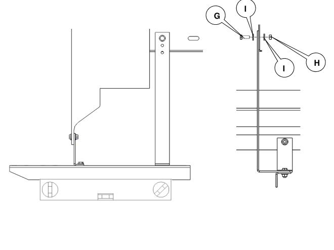
At the rear Driver's Brace Location (Marked as 2 on the Diagram), use a Frame Bracket (D) and attach to the Angle Brace using one 1/4"-20 X1" Bolt (G), two 1/4" Washer (I), and one 1/4"-20 Nut (H) using a 7/16" Wrench or Ratchet. Do not completely tighten at this time.
