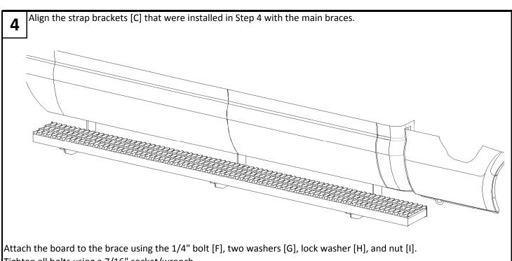
Tighten all bolts using a 7/16" socket/wrench.
