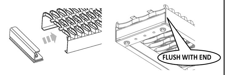
DO NOT INSTALL THE END CAP ON THE OTHER END OF THE BOARD UNTIL COMPLETING THE NEXT STEP.
