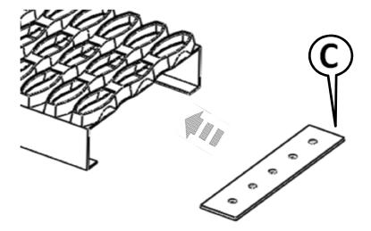
Once the strap brackets are in the board, attach the other end cap.
