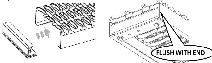
DO NOT INSTALL THE END CAP ON THE OTHER END OF THE BOARD UNTIL COMPLETING THE NEXT STEP.
