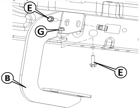
For the crew cab middle brace location, the other top slot will be used to attach the brace.
