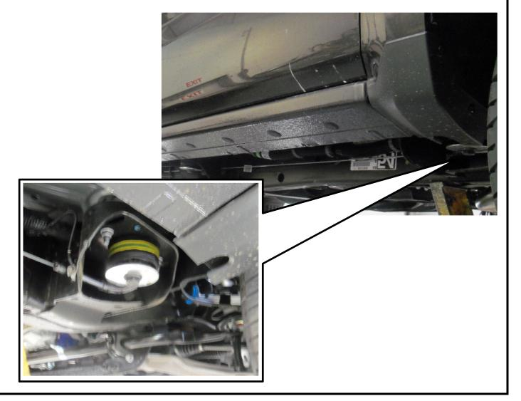
Remove the bolt from the body shock mount at each of the mounting locations using a 21mm socket.
