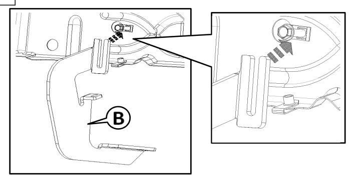
Attach the bottom mounting location using the 8mm bolt [E].
