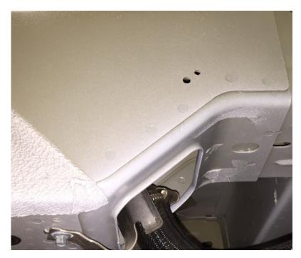
At the front Passenger's Brace Location (Marked as 3 on the Diagram on Page 5), use a Frame Bracket (E) and attach to the tube running lengthwise of the vehicle using one 8mm Small Threaded Plate (K) and one M8-20mm Hex Head Bolt (J). Insert the M8 bolt (J) through the side with the single hole and attach the 8mm Small Threaded Plate (K) as shown in the picture below. While pulling down on the brace, tighten the M8 bolt J) using a 13mm Wrench or Ratchet. Do not completely tighten at this time.
