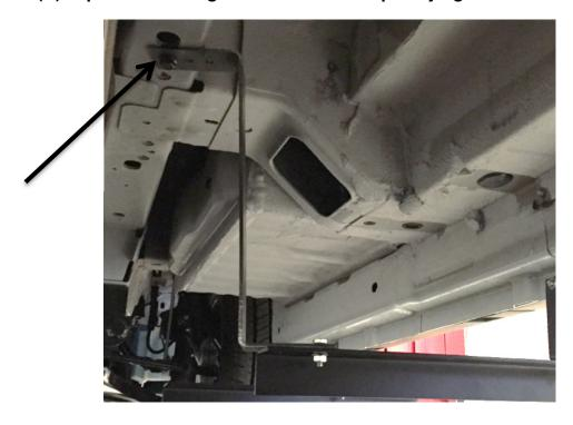
14 Slide two Strap Brackets (F) into the Running Boards (A).
