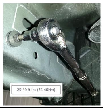
Put a 8mm x 25mm bolt [F] through the top hole in the braces and thread into the 8mm threaded plate [G] until the bolt starts to come through the threaded plate.
