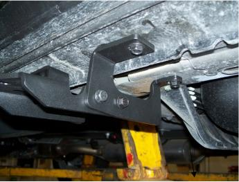
Place running board (A) onto the brackets. Align 8mm square head bolts (H) in the bottom of the running board (A) with holes in the brackets. Completely tighten brackets to vehicle. Center board on vehicle between wheel well openings or until desired appearance is aquired. Adjust board in/out on vehicle until desired appearance is met. Secure board into palce using 8mm hex nuts (L).
