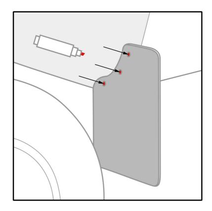
Step 2 Align flap to desired height.
