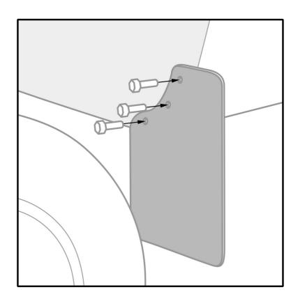
Step 3 Drill 3 holes through the flap and wheel well lip and attach with 1/4" screws.
