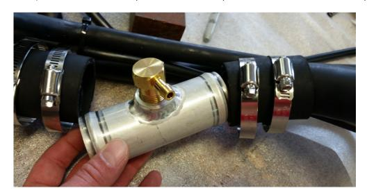
8) Secure the fill line adaptor with the large hose clamps.
