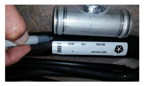
4) Place some type of barrier between the steel fuel line and the other smaller lines so that they are not accidentally cut.
