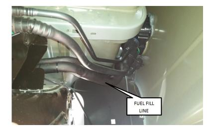
Check your vehicles fill line to insure you have the correct kit before starting installation.
