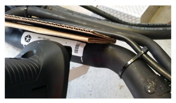
6) Place a 2.5" large hose section and 2 large hose clamps on each end of the fill line.
