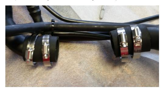
7) Install the fill line adaptor as horizontal as possible, with the roll over valve upright.
