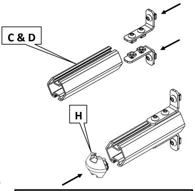
Install endcaps (H) on the tubes (C&E) by first hand pushing them to set in place, then hitting them with a rubber mallet.
