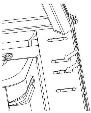
Should your Cab Rack not have any of the available slots line up with the stake pocket holes, or the available slots do not allow the rubber mounting block to insert properly, drill a hole into the Cab Rack Mounting Plate to properly line up with the stake pocket hole.
