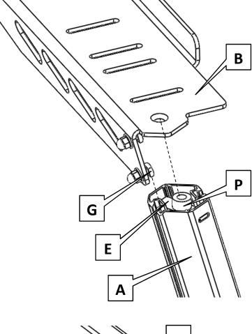
Align **(P)** 3/8-1.25" Flat Socket Bolt with the countersunk hole in **(B)** Left Bolt-On Brace ensuring **(P)** 7/16" x 1/2" Nylon Spacer stays in place on top of the Threaded Plate. Tighten Hardware.
