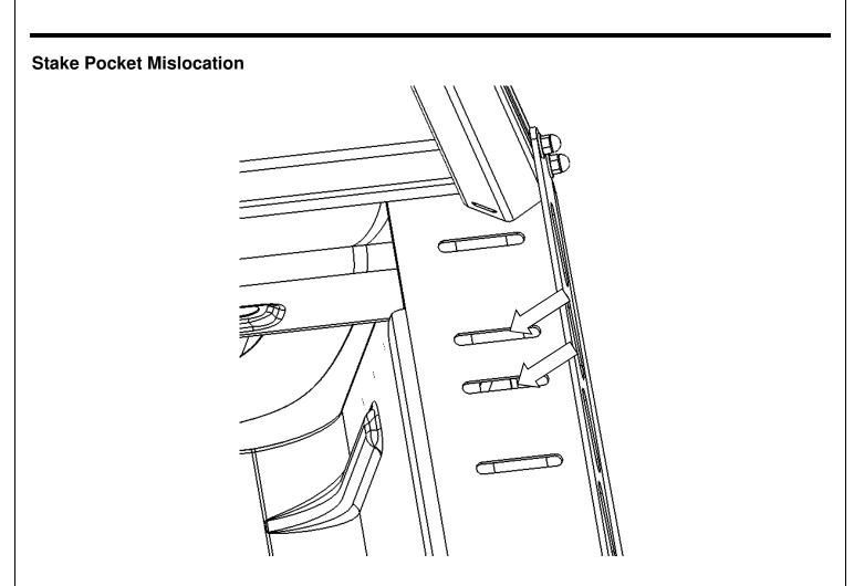
Should your Cab Rack not have any of the available slots line up with the stake pocket holes, or the available slots do not allow the rubber mounting block to insert properly, drill a hole into the Cab Rack Mounting Plate to properly line up with the stake pocket hole.
