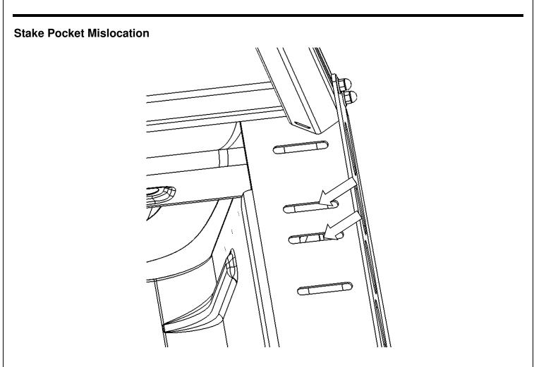
Should your Cab Rack not have any of the available slots line up with the stake pocket holes, or the available slots do not allow the rubber mounting block to insert properly, drill a hole into the Cab Rack Mounting Plate to properly line up with the stake pocket hole.
